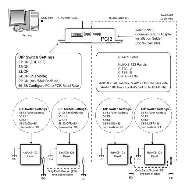
Figure 17: RS-485 Connection via PCI-3 with Multidrop Panels at Both Ends
